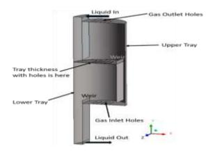
Figure 1 Model geometry and boundaries of the circular cross-section sieve tray (the plane of symmetry is just the whole front face of geometry shown, towards +z direction shown)
