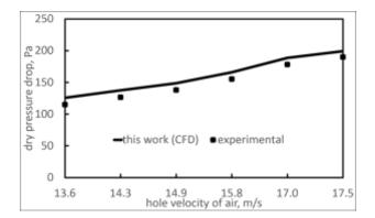
Figure 6 Dry pressure drop of circular cross-section sieve tray
