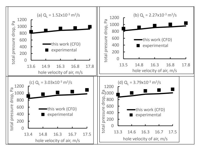
Figure 5 Total pressure drop of circular cross-section sieve tray
