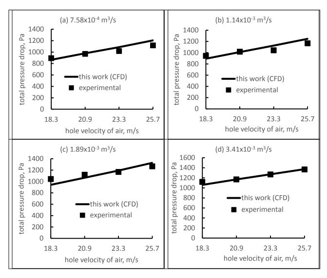
Figure 7 Total pressure drop of rectangular cross-section sieve tray
