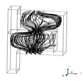
Figure 10 Gas streamlines (in dark black) of the two phase flow (water flow rate =  $3.41 \times 10^{-3}$  m<sup>3</sup>/s, air hole velocity = 25.7 m/s, rectangular tray)
