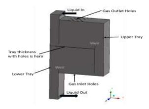
Figure 2 Model geometry and boundaries of the rectangular cross-section sieve tray (internal features are not visible and shown)
