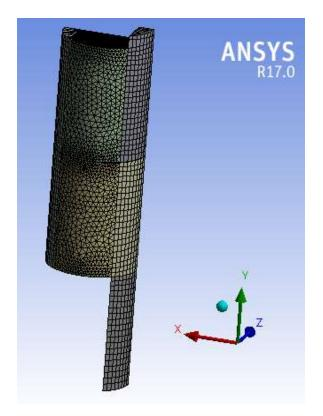
Figure 3 Mesh of circular cross-section sieve tray model geometry
