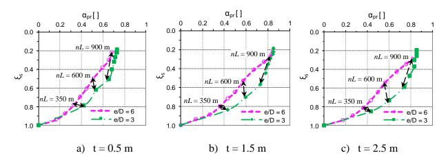
Fig. 7 Variation of the normalized settlement with pile-raft coefficient for different geometric conditions
