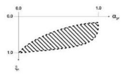
Fig. 1 Relationship between normalized settlement and pile-raft coefficient [4]
