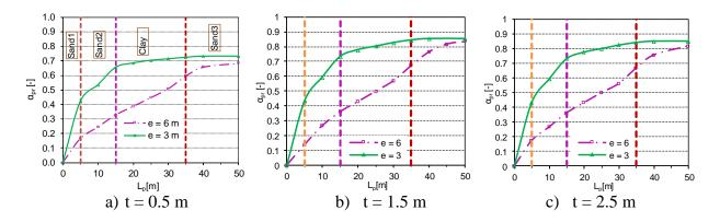
Fig. 6 Variations of the pile raft coefficient with geometric parameters of the piles and raft.
