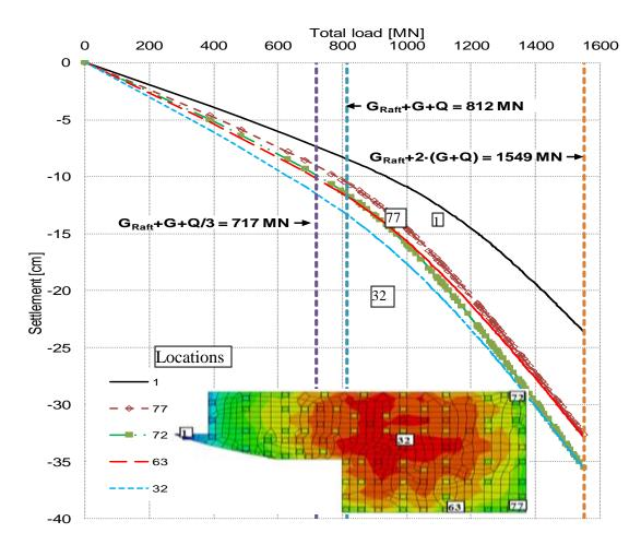
Fig. 8 Load settlement curves at different locations
