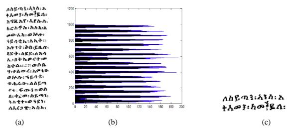
Figure 7: Line segmentation error (a) input image (b) Y histogram (c) error segmented
