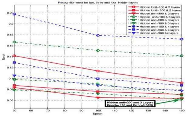
Figure 10: Graph of overall recognition error with two, three and four layers
