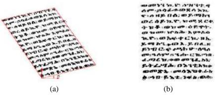
Figure 5: Output of skew detection: (a) skewed image (b) deskewed image
