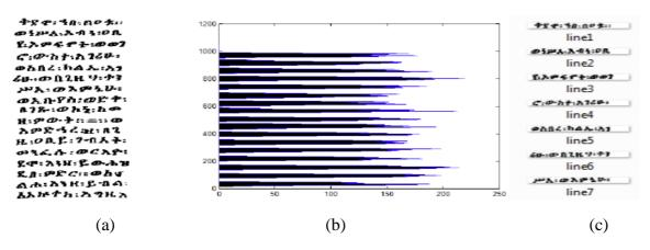
Figure 6: Output of line segmentation (a) input image (b) Y histogram (c) segmented line
