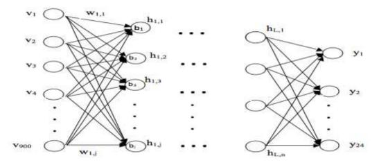
Figure 2: Architecture of the proposed deep network with 900 input, L hidden and 24 nodes of layers
