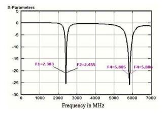
Figure 10: 3dB band width of dual band F shape antenna at 2.45 and 5.8 GHZ
