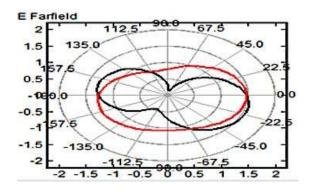
Figure 12: Far field radiation pattern (linear).
