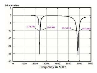
Figure 9: -10 dB band width of dual band F shape antenna at 2.45 and 5.8 GHZ
