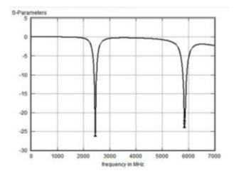
Figure 3: S-Parameter versus frequency for dual band inverted L micro strip antenna.
