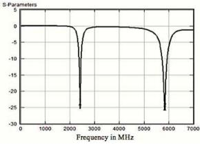
Figure 8: S-parameter versus frequency for dual band F shape microstrip antenna
