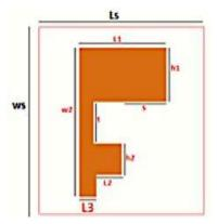
Figure 2: F-antenna geometry at 2.45 and 5.8 GHz.
