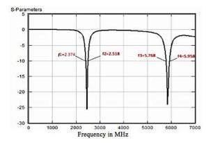
Figure 4: -10dB bandwidth of dual band inverted L antenna at 2.45 and 5.8 GHz.
