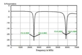
Figure 5: 3dB bandwidth of dual band inverted L antenna at 2.45 and 5.8 GHz.
