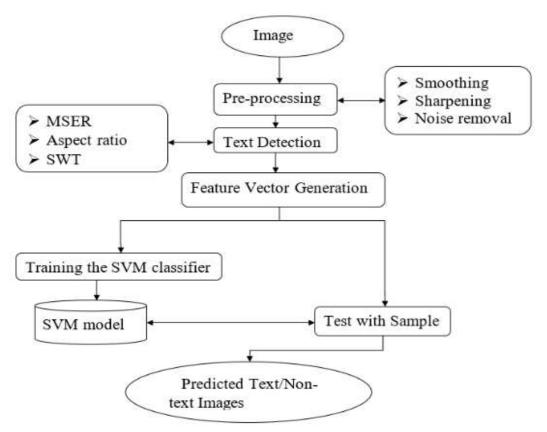
Fig. 1: System architecture for text detection
