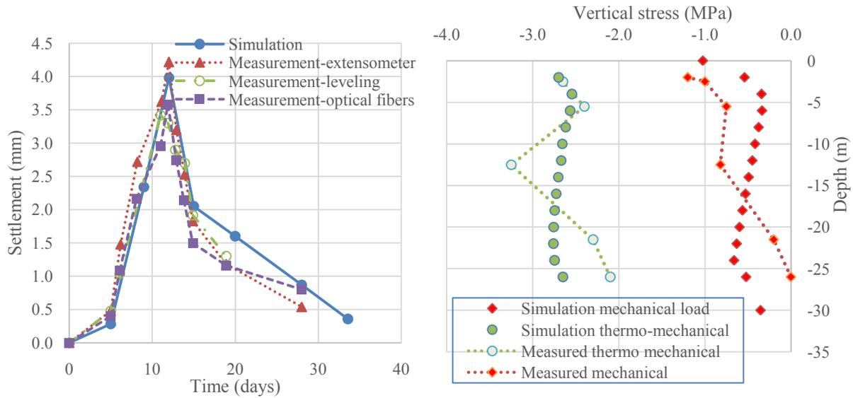
a) Settlement versus time(1<sup>st</sup> cycle)                      b) vertical stress with depth (7<sup>th</sup> cycle)
