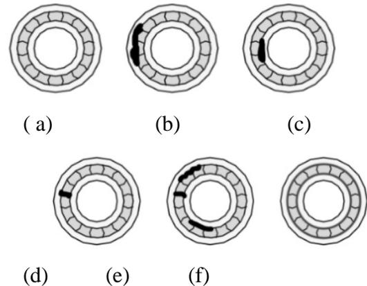
**Figure 3** Types of faults and their locations; a) healthy bearing, b) damage on outer race, c) damage on inner race, d) damage on roller body, e) damage on roller body, outer and inner race, f) heavily worn bearing
