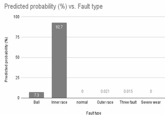
**Figure 7** Inner race fault Prediction on second round data
