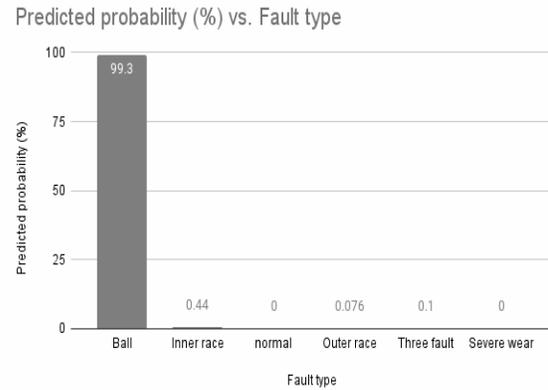
**Figure 6** Ball fault Prediction on second round data
