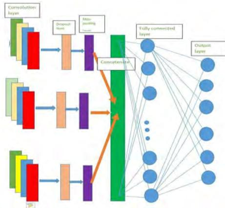
Figure 4 Proposed CNN architecture for 6 classes
