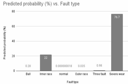
**Figure 11** Severe wear fault prediction
