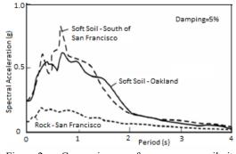
Figure 2 Comparison of average soil-site spectra in Oakland and San Francisco areas with average rock-site spectra in the region during 1989 Loma-Prieta earthquake [16,17]
