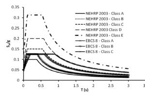
Figure 9 Comparison of EBCS 8 spectra and NEHRP spectra adapted to a return period of 100 years for Zone 2 (including Addis Ababa)
