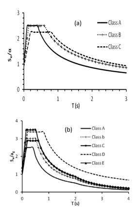
Figure 7 Normalized elastic response spectra: (a) EC 8: 1994 [7]; (b) EC 8: 2004 – Type 1 (for  $M_s \ge 5.5$ ; re-plotted after [8])
