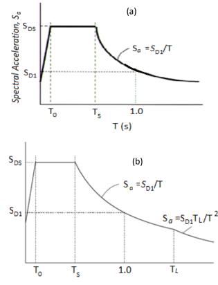
Figure 6 The basic design spectral curves according to (a) NEHRP 1997 [3]; (b) NEHRP 2003[4]
