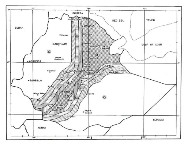
Figure 11 Seismic hazard map of Ethiopia for 100-year return period as per EBCS 8: 1995 [23]
