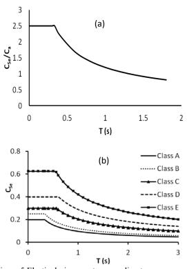
Figure 5 Elastic design spectra according to NEHRP 1994 (a) Basic [2]; (b) For  $A_a=A_v=0.1$
