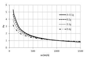
Figure 4 Variation of spectral amplification factors versus  $v_s$  for short and long period ranges
