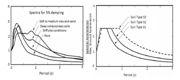
Figure 1. (a) response spectra for different site conditions after Seed et al [12]; (b) The design spectra proposed by ATC-3:1978 Project [16,17]
