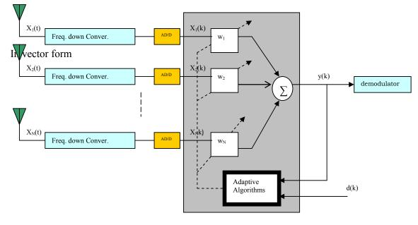
Figure 1 Block diagram of an adaptive array antenna.
