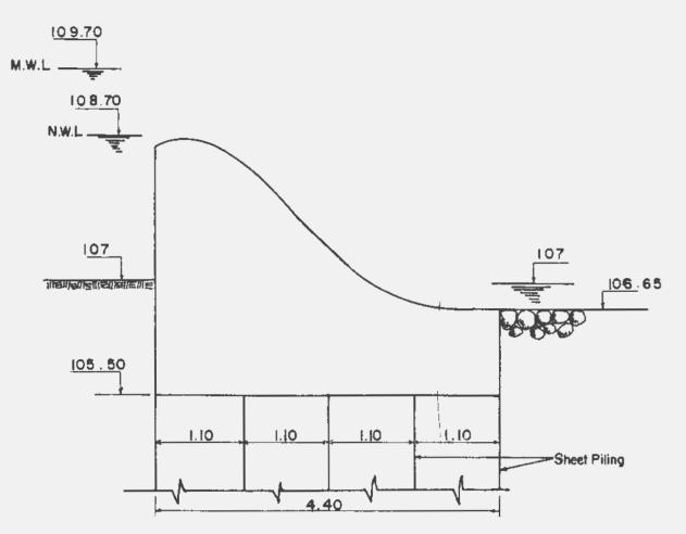
Fig. 1 — Preliminary Design of the Diversion Dam
