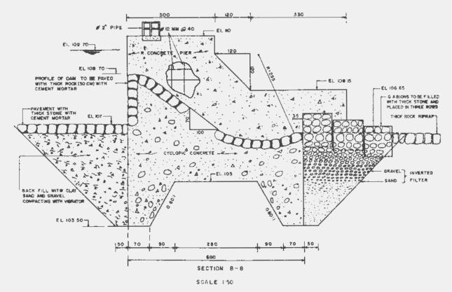
Fig. 6 — Final design of the Diversion Dam
