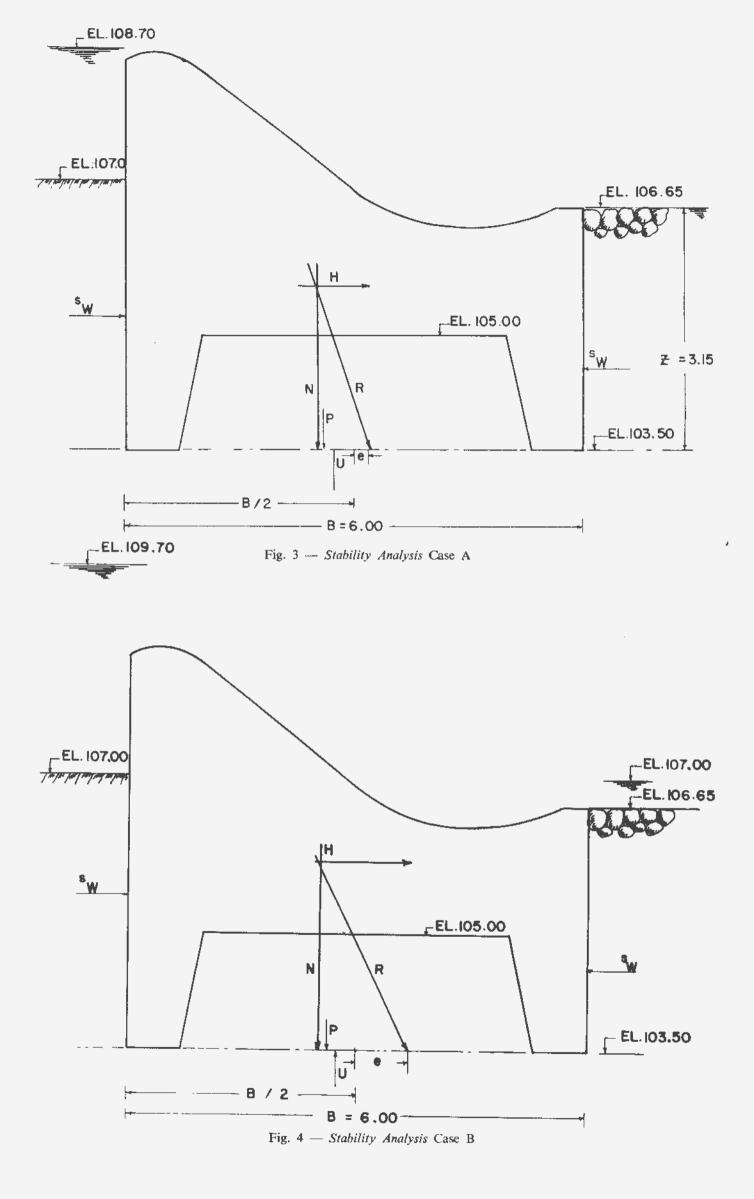
On the basis of the results of the foregoing analysis the following elements have been fixed for the final design of the diversion dam (Figs. 3 & 4)
