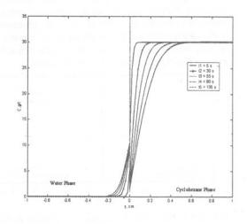
Figure 10 Concentration profiles at the inter phase with one-dimensional diffusion equation for mass transfer with chemical reaction.
