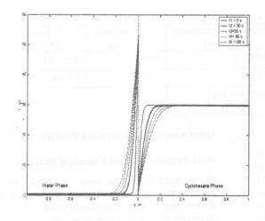
Figure 8 Analytical solution of concentration profiles at the inter phase with onedimensional diffusion equation for mass transfer without chemical reaction.
