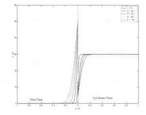
Figure 7 Numerical simulation of concentration profiles at the inter phase with onedimensional diffusion equation for mass transfer without chemical reaction.
