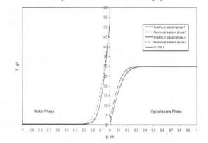
Figure 6 Comparison of concentration profiles at the inter phase with one-dimensional diffusion equation for mass transfer without chemical reaction with an analytical solution.
