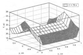
Figure 13 Temperature profiles at the inter phase with two-dimensional equation for mass transfer with chemical reaction. The water phase is in the negative and the Cyclohexane phase is in the positive side of the axis.
