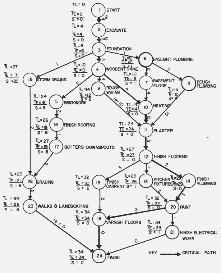
Fig. | CRITICAL PATH DIAGRAM
