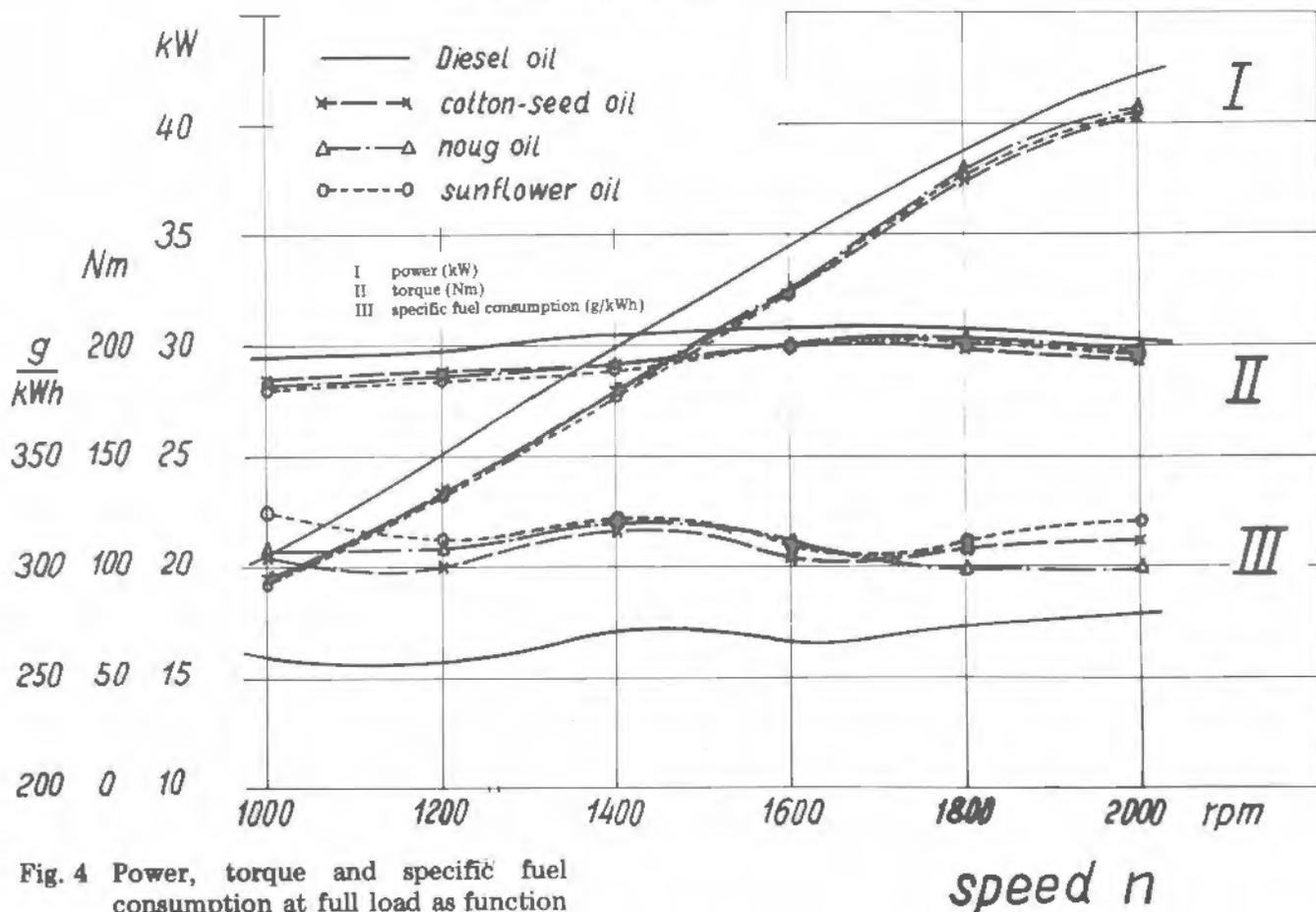
Fig. 4 Power, torque and specific fuel consumption at full load as function of the speed. Comparison between non-esterified vegetable oils and diesel oil
