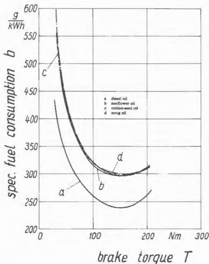
Fig. 2 Specific fuel consumption as function of the brake torque at 1600 rpm. Comparison between non-esterified vegetable oils and diesel oil
