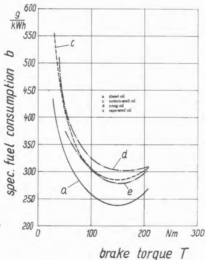
Fig. 3 Specific fuel consumption as functions of the brake torque at 1600 rpm. Comparison between esterified vegetable oils and diesel oil
