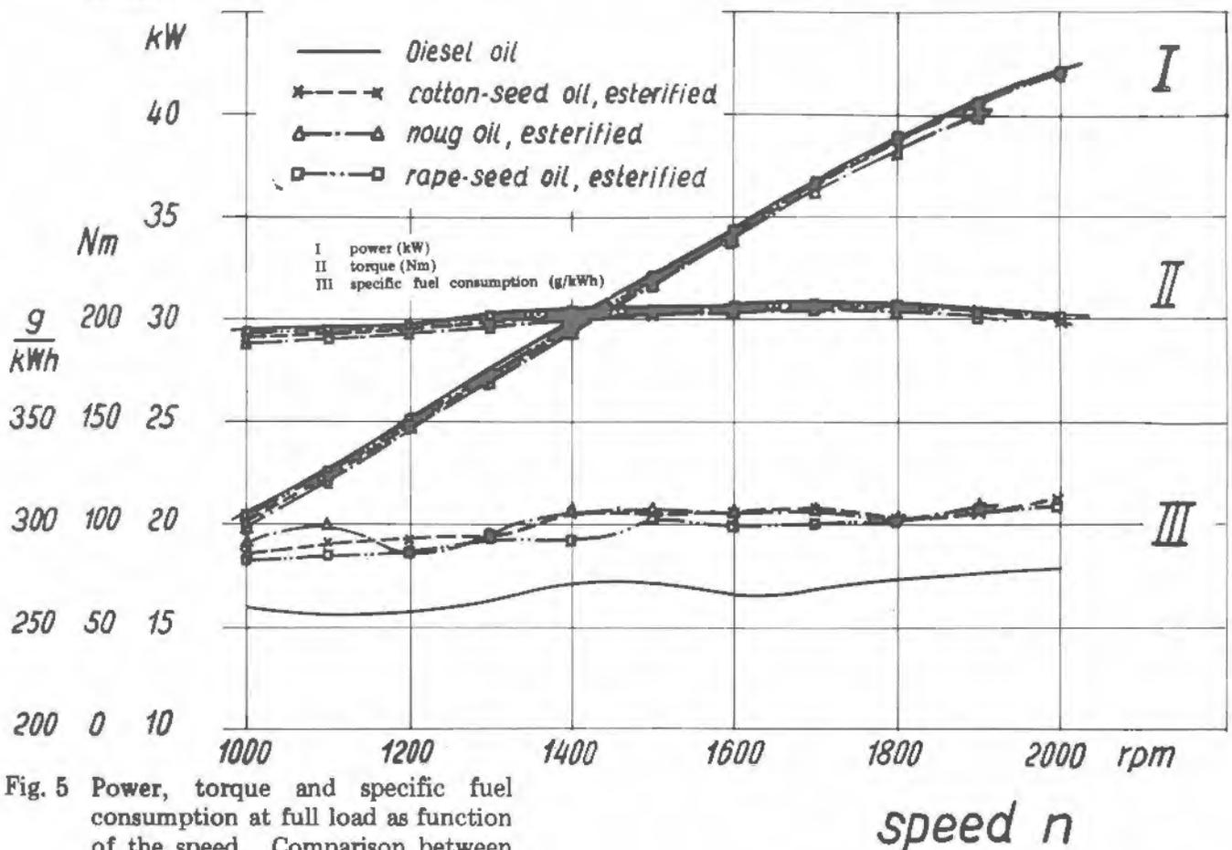
Fig. 5 Power, torque and specific fuel consumption at full load as function of the speed. Comparison between esterified vegetable oils and diesel oil.
