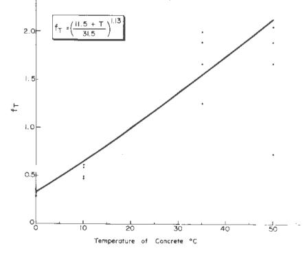
Fig. 2. Maturity Function for Calculating Equivalent Curing Age at  $20^{\circ}C$ .
