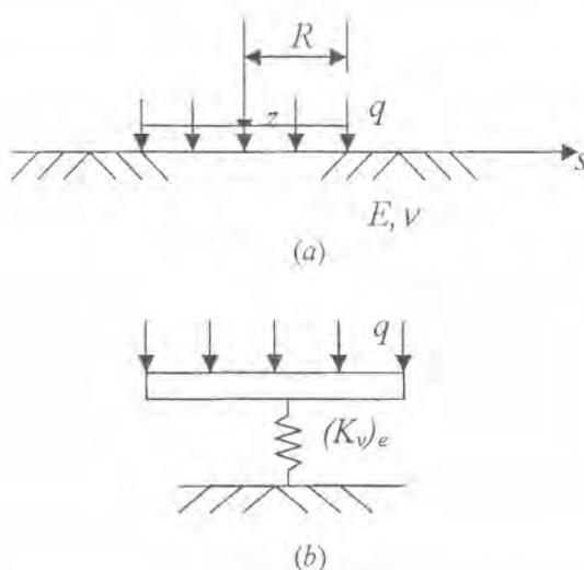
Figure 1 (a) An ideally flexible circular footing on the surface of an elastic half space;
