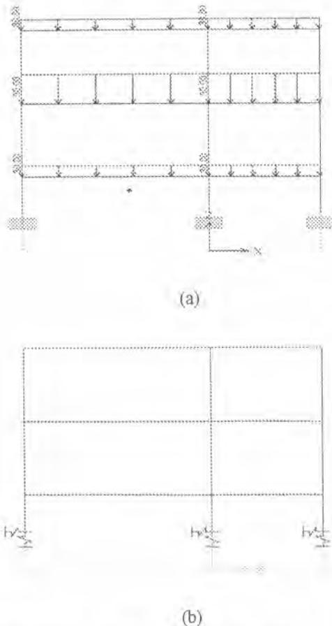
Figure 5 (a) The fixed-base frame with the loading; (b) The flexible-base frame
