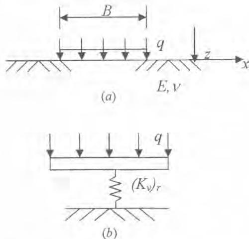
Figure 2 (a) An ideally flexible rectangular footing on the surface of an elastic half space; (b) A model of the rectangular footing supported by a linear spring
