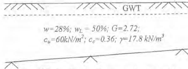
Figure 6 Idealized stratification of the soil formation
