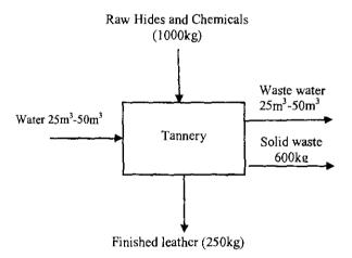
Figure I Schematic diagram for inputs and outputs of a typical leather industry
