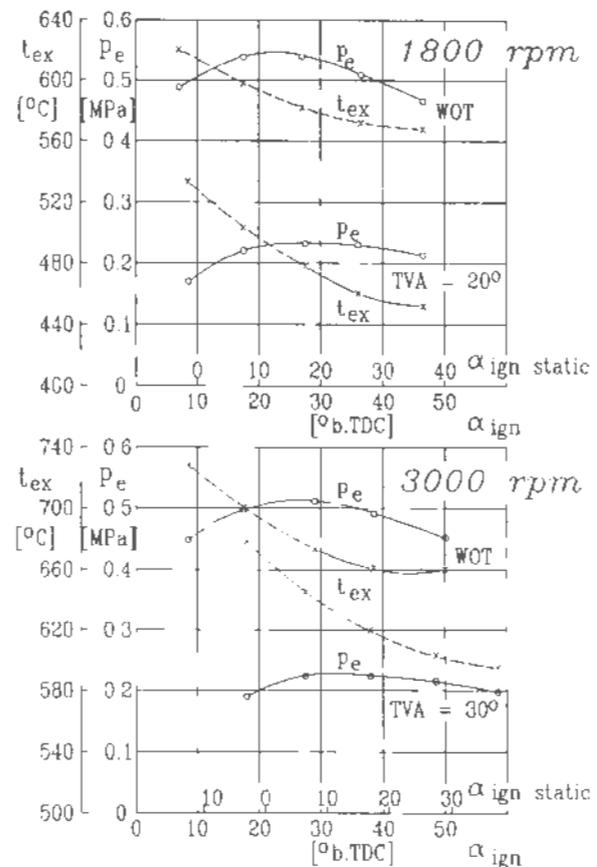
Figure 8 Optimization of Ignition Timing of VW Boxer Engine
