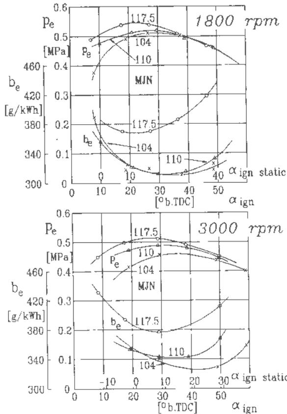
Figure 9 Full Load Optimization with Different Main Jets
