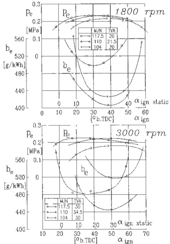
Figure 10 Part Load Optimization with Different Main Jets
