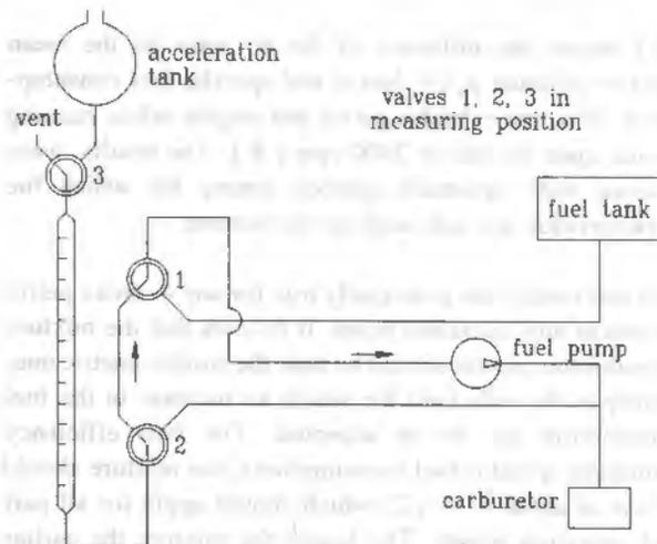
Figure 4 Fuel Consumption Measuring Device
