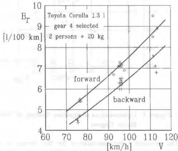
Figure 5 Road Fuel Consumption with Changed Velocity
