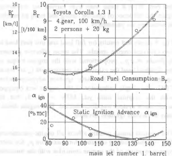
Figure 7 Optimum Road Fuel Consumption
