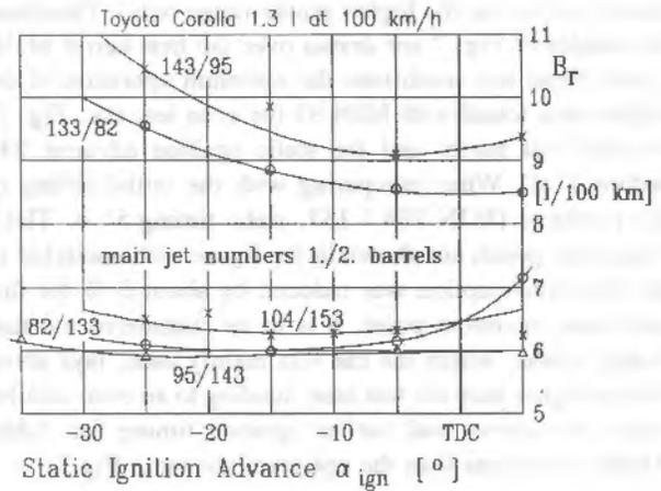
Figure 6 Optimization of Main Jet and Timing
