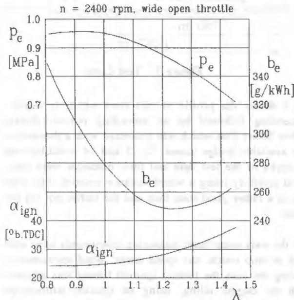
Figure 1 Air Ratio Influence in Engine Parameters
