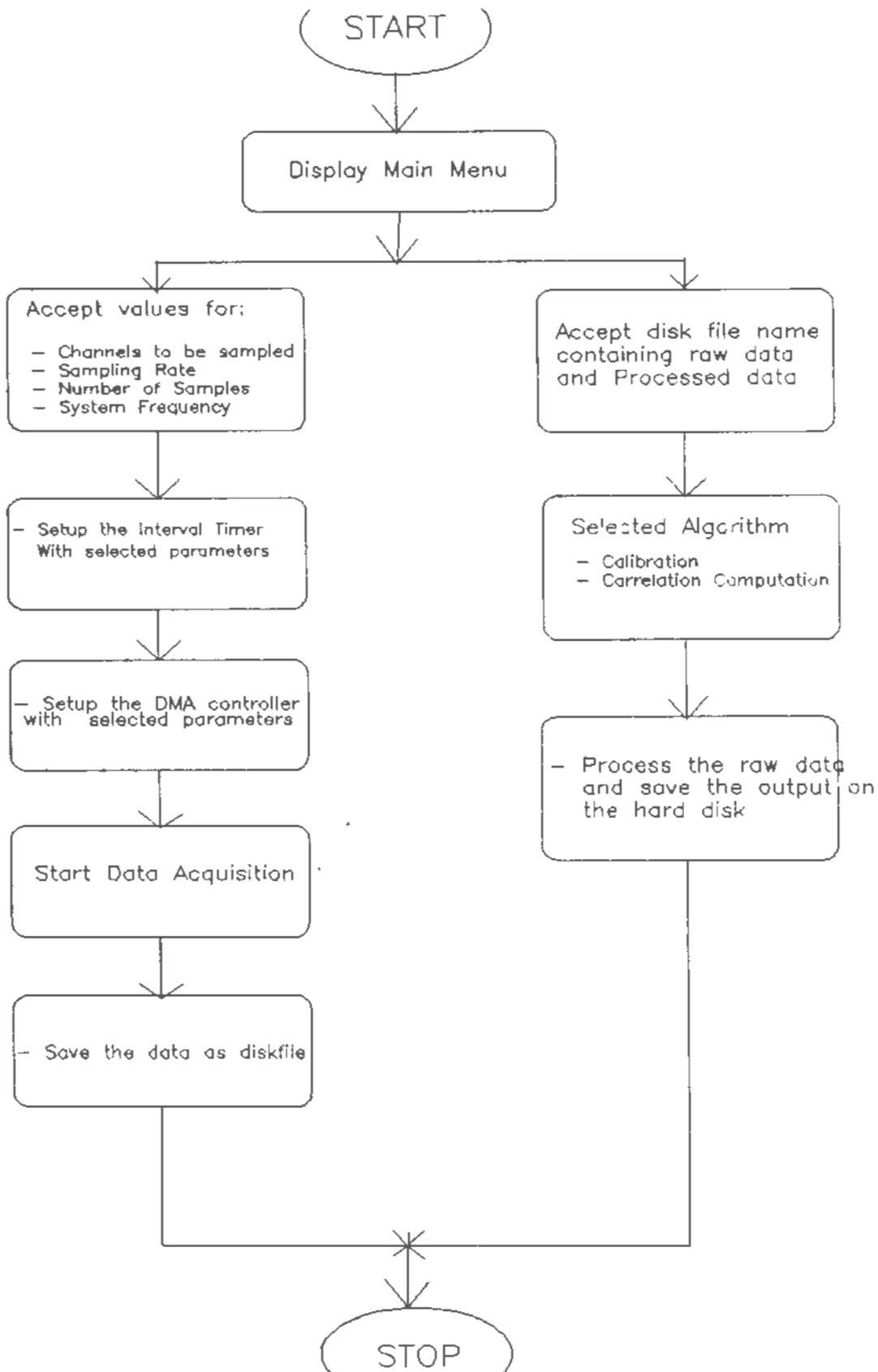
Figure 1.2 Flow Chart of the Driver Software
