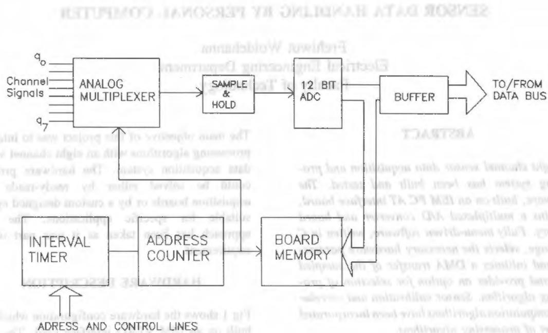
Figure 1 Block Diagram of Interface System
