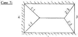
Figure 9 Slab panel simply supported along one of the shorter sides only.
