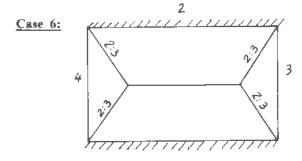
Figure 8 Slab panel continuous along the two shorter sides only
