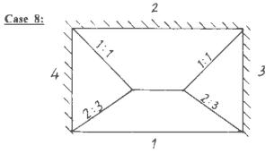
Figure 10 Slab panel simply supported along one of the longer sides only
