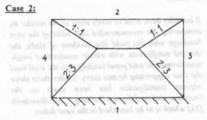
Figure 4 Slab panel continuous along one of the longer sides only.
