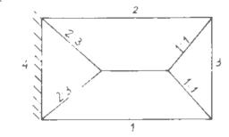
Figure 5. Slab panel continuous along one of the shorter sides only.
