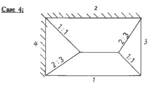
Figure 6 Slab panel continuous along the two adjacent sides only
