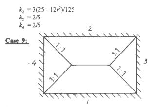
Figure 11 Slab panel continuous along all four sides
