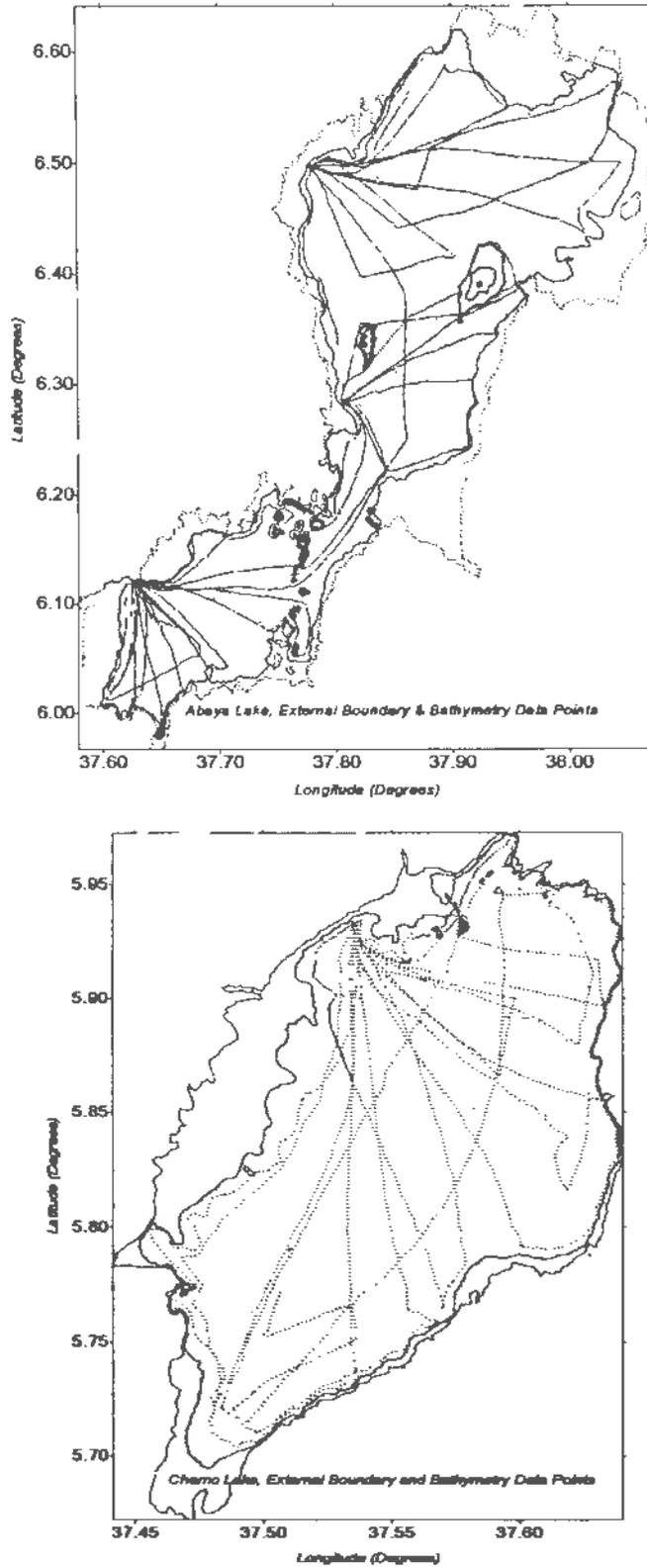
Figure 3 Abaya and Chamo lakes Bathymetry Survey Points, Boundary and Captured External Contour Line
