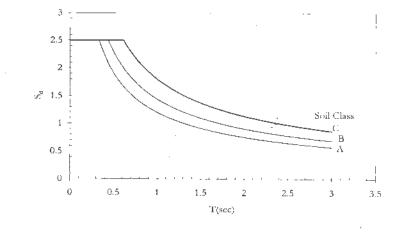
Figure 4: The design spectra of EBCS 8 for the ESF method of analysis for a bedrock acceleration ratio of,  $\alpha = 1$ , common occupancy structure (*I*=1), and an elastic response of the structure ( $\gamma$ =1)
