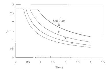
Figure 1 The design spectra of UBC 94 for l=1,  $R_w=1$  and a base shear coefficient normalized with respect to the zone factor
