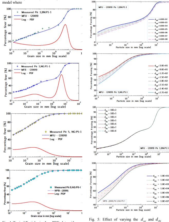
Fig. 4: Typical Particle size Log-PDF plots with experimental and best fit curves using MFU - (2009) and MFB - (2009)
