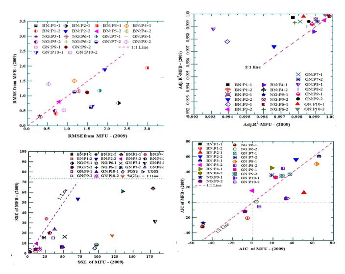
Fig. 3: Statistical Goodness Fit Comparison between Unimodal and Bimodal MF - (2009) Models using Control PSD Data.
