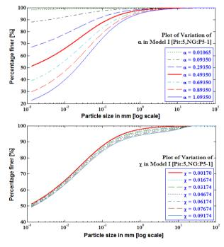
Fig. 10.Effect of varying the  $\alpha$  and  $\chi$ parameter for Model-I, unimodal fit for Pit:5,NG:P5-1:
