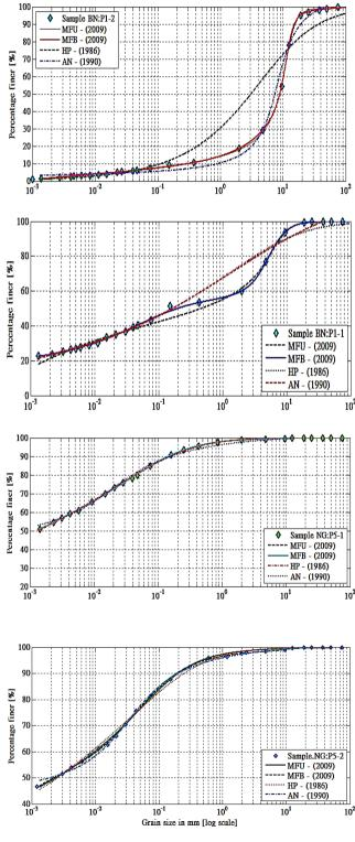
Fig. 2: Typical experimental data fitted using the four PSD models for soils of different gradation
