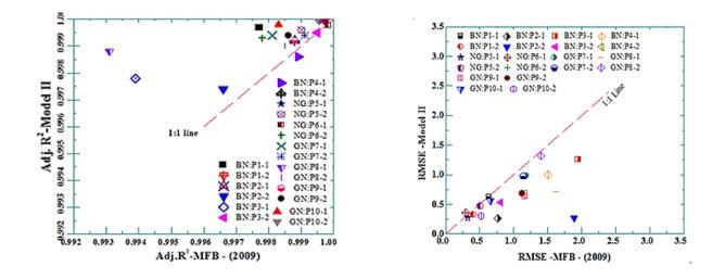
Fig. 13: Statistical Goodness Fit Comparison between Model-II (New Bimodal model) and MFB - (2009) models using control PSD data
