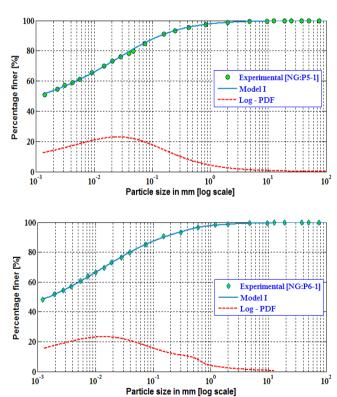
Fig. 8: Typical particle size Log - PDF plots with experimental and best fit curves using Model-I (unimodal model) for various textured soils (Pit 5, NG: P5:1).and (Pit 6, NG: P6:1).
