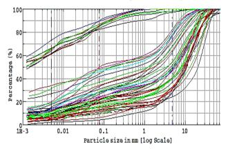
Fig. 1: Particle-size distribution test data on TWR soils used for analysis.
