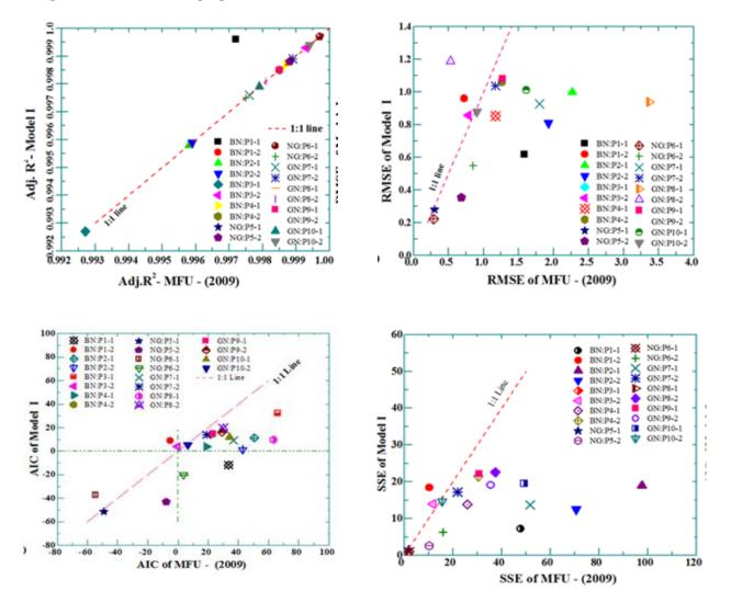
Fig. 6: Statistical Goodness Fit Comparison between Model-I (New unimodal model) and MFU - (2009) models using control PSD data
