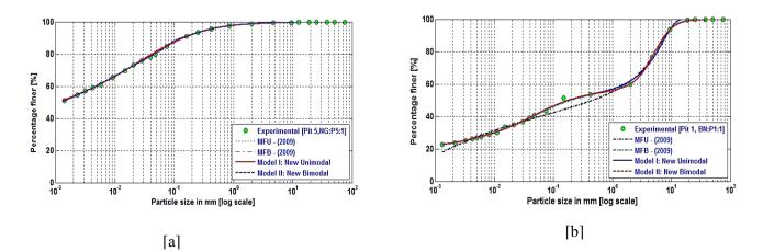
Fig. 17: Comparison of experimental, MFU - (2009), MFB - (2009), Model-I (New unimodal) and Model-II (New bimodal) models fitted totypical:
